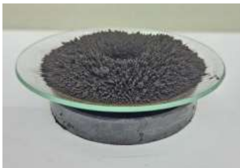
Figure 2 Prepared magnetite-activated carbon-clay Composite
